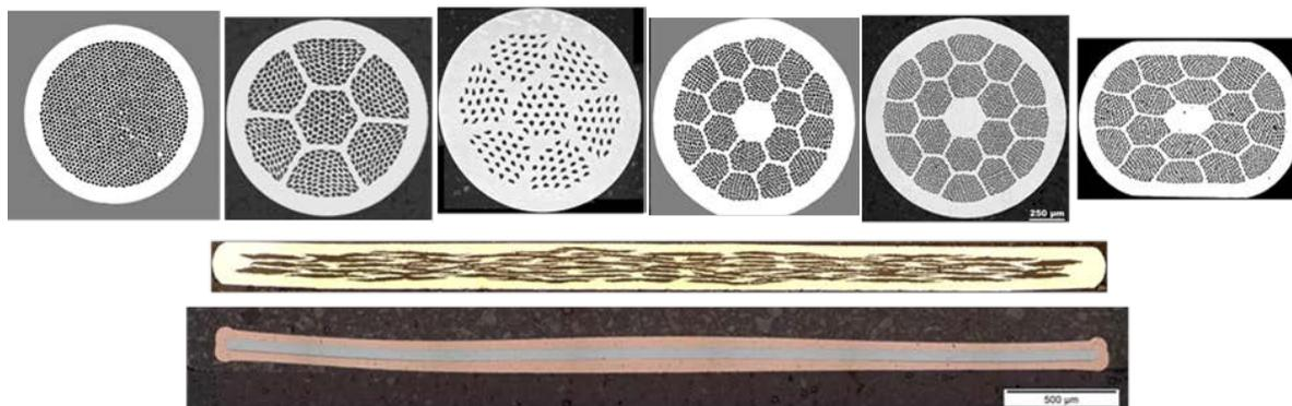
Top row shows various Bi-2212 wires displaying a wide variety of filament architectures. Note the very strong contrast with the Bi-2223 flat tape (~0.2 x 4 mm – middle row) made by Sumitomo Electric Inc. in only one single architecture and the flat SuperPower REBCO coated conductor (bottom row) made for the NHMFL 32 T user magnet (~0.14 x 4 mm).
