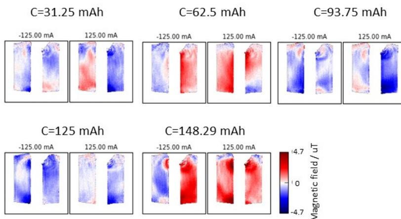
Figure 2. Magnetic field generated by the current inside the battery while the cell was being charged and discharged at 100 mA at different state of charge
