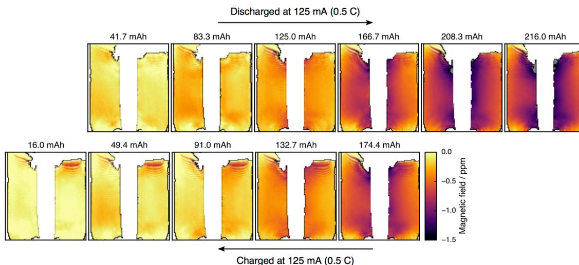
Figure1. Magnetic Resonance Image of the medium around the battery at different state of charge of the battery.
