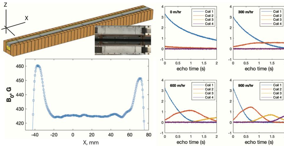
**Fig. 1.** **Left:** magnet and coil structure; The magnetic field at the sweet spot  $\sim 3.8$  cm above the coil surface is uniform along the X direction within  $\pm 1.2$  G for 70-cm length. The B1 field from all coils were adjusted to be uniform ( $\pm 10\%$ ) over the entire 4 coils. Each coil is 17 cm long. **Right:** Signals from a 13-cm long sample starting from Coil 1.
