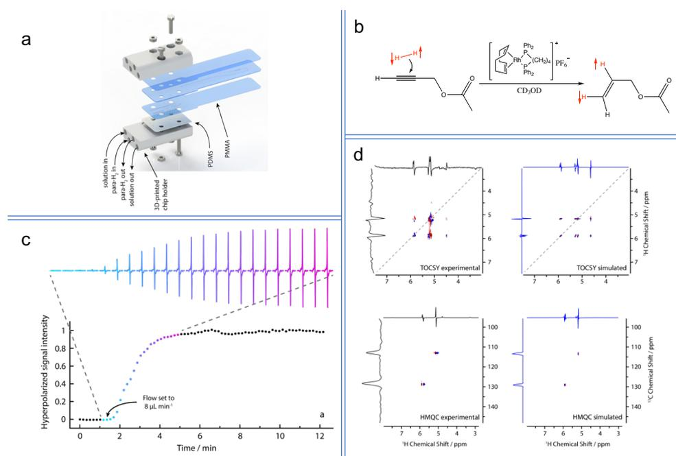
Fig 1 a) chip assembly b) scheme of the hydrogenation reaction c) build-up of the hyperpolarised signal d) experimental (black) and simulation (blue) 2D NMR spectra of the hyperpolarised reaction mixture.
