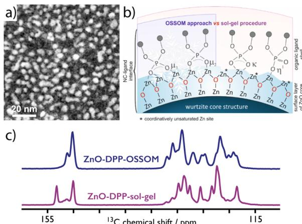
**Figure 2.** Zinc oxide nanocrystals (STEM in (a)) with diphenylphosphate ligands (schematic in (b)) prepared using different synthetic procedures display contrasting organic-inorganic interfaces (via <sup>13</sup>C NMR spectra (c)).
