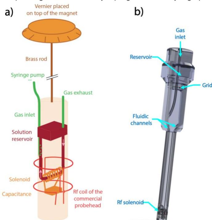
**Figure 1.** a) Principle of the WIFI-NMRS device
