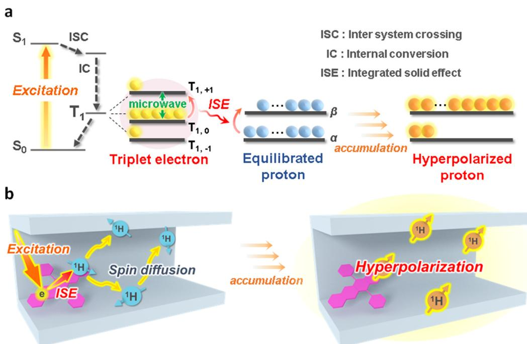
**Fig. 1** (a) Typical scheme of Triplet-DNP. (b) Schematic illustration of Triplet-DNP in MOFs accommodating polarizing agents.
