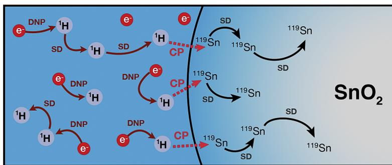
**Figure 1.** Pulsed cooling of powdered  $\text{SnO}_2$ . Hyperpolarization is generated on  $^1\text{H}$  nuclei in a wetting phase and transferred to  $^{119}\text{Sn}$  nuclei at the surface of the material with repeated cross-polarization contacts. Slow spin diffusion between tin nuclei transports the polarization towards the bulk.
