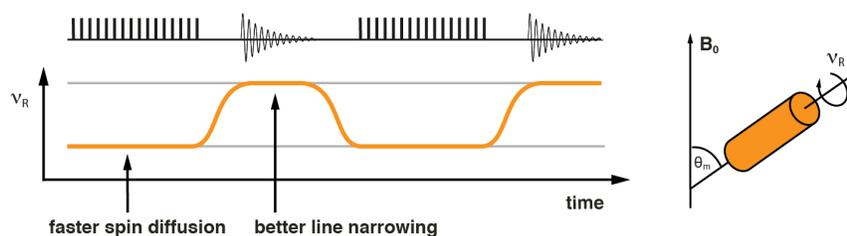
**Figure 2.** Schematic representation of how the MAS rate is modulated during the experiment. Hyperpolarization and spin diffusion towards the bulk happen at a slow spin rate. The MAS rate is then increased before acquisition of the FID.
