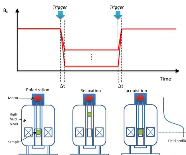
Figure 1: Scheme of shuttle NMR
