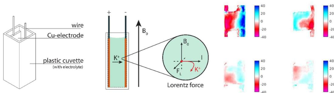
Figure 1. Left: Design of the electrochemical cell and observable effect. Right: Out of plane velocities (mm/s) of a cuvette filled with salt water at different currents measured utilizing FLIessen. The electrodes are attached to the cuvette walls (top/bottom in the images). Top row: +/- 20 mA; Bottom row: +/- 5 mA.
