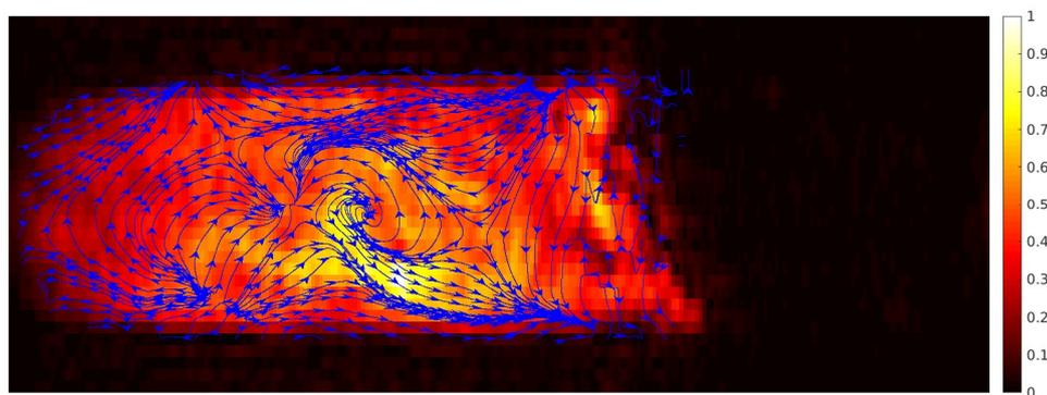
Figure 2. Streamline plot of a cuvette cell filled with a 1M  $\text{CuSO}_4$  solution measured with spin echo velocity imaging. The plane is parallel to the electrode plates. In the background, the spin density is depicted.
